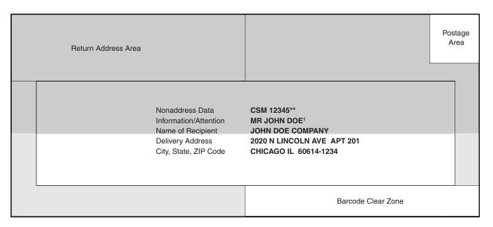
1. For MLOCR *FASTforward* users, the name of the recipient must appear in the OCR read area. Dark shaded area indicates "free space" for nonaddress printing. Light shaded area indicates preferred clear zone to enhance readability.
